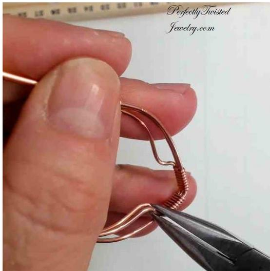
Because your heart stone is not 'flat', you will need to make some room in the wires for the stone. Use your fingers and gently spread out the wire tabs.
