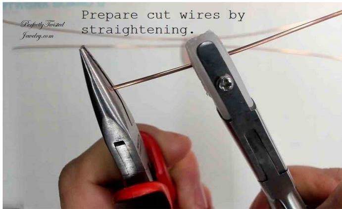
Prepare cut wires by straightening.
